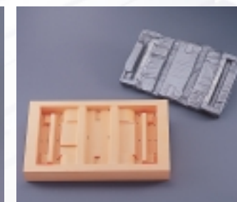
A poured plastic part produced from a mold milled in chemical wood
