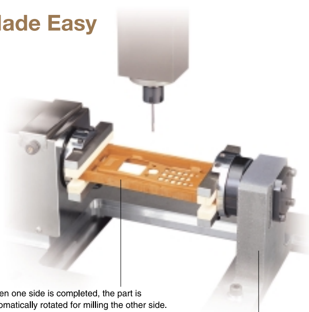
Adjustable holders secure the material being milled.
