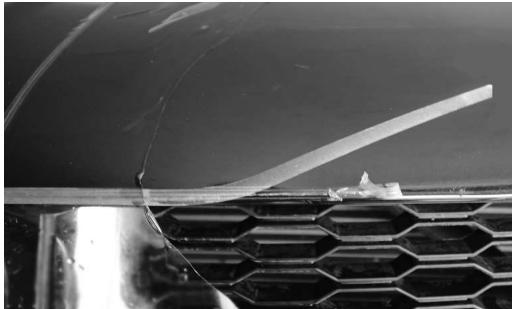
5. **With a 6-8 inch lead angled away from the Knifeless Tape lead, apply cover tape over film and knifeless tape, covering 2-3 inches of the Knifeless tape lead and tail (starting at an angle and leaving at an angle).**
