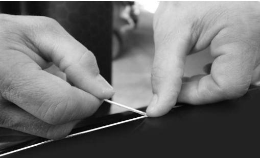
2. Start all lines (both lead and tails), by folding the start of the tape back over itself approximately 3 inches. Press thumb firmly on folded edge, covering at least 1/2 inch of tape.
