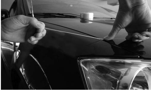
1. Begin with 6-8 inches of tape (before and after) where the film will be cut and lay down Knifeless Tape. Apply tape everywhere film will be cut.
