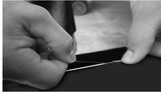
3. Firmly grasp the end of the tape with your thumb and index finger, positioning your two thumbs close together to start the filament. Gently pull the line to tear the carrier tape and expose the filament. Pull the filament back and not upward, 2 inches. Tack end of filament to vehicle until ready to cut film.
