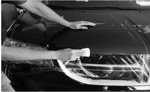
4. **Apply the film over the tape, leaving the lead and tail tape visible, according to wet application instructions.**
